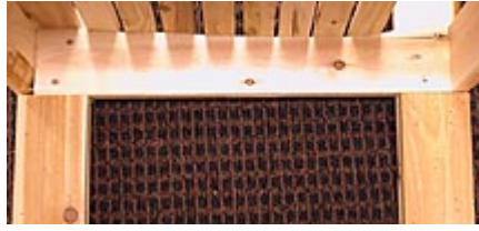
The upright connector with seat slats already installed.
